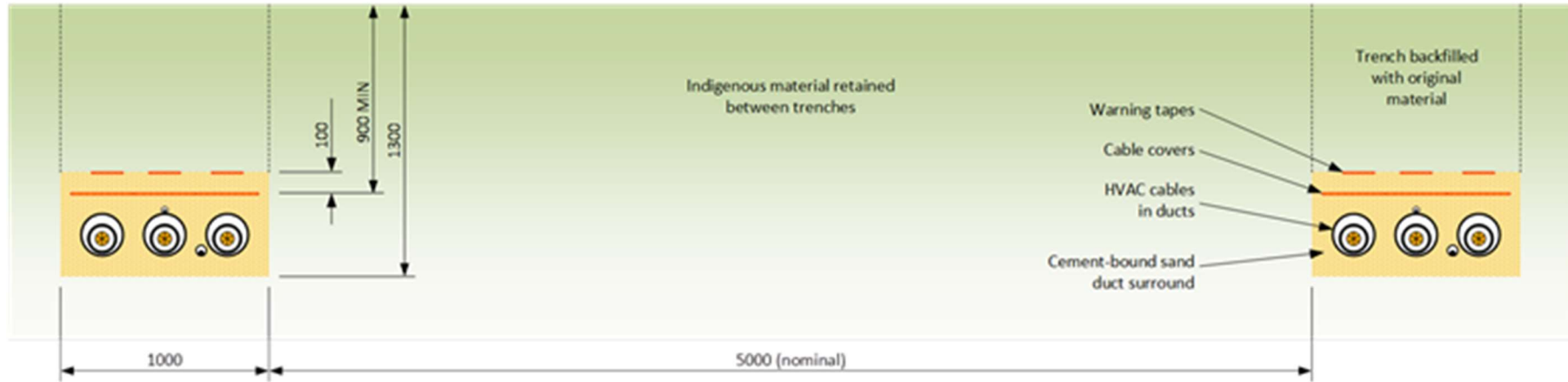
Plate 3.5 - Typical arrangement of HVAC cables and FOC in ground (all measurements in mm).
